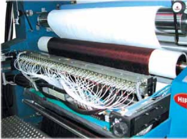
integrated of HIP-MITSU dispenser for hot melt adhesive
