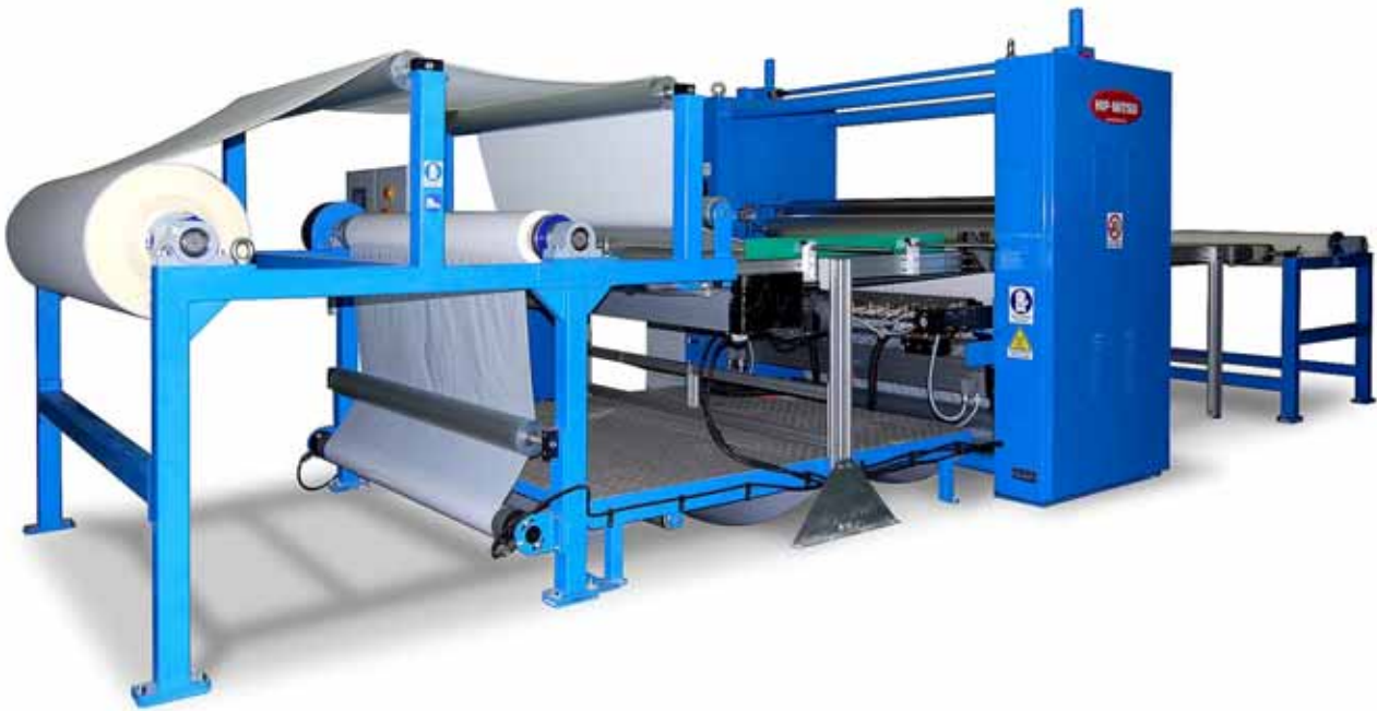
example of converting line for material in roll and in sheet, included of motorized belt, suitable for foam, textiles, nonwoven, silicon paper and film, and more ...
