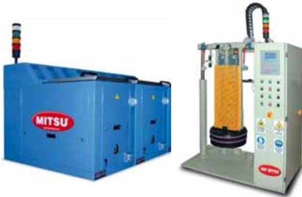
tank and drum melter, pumping station
