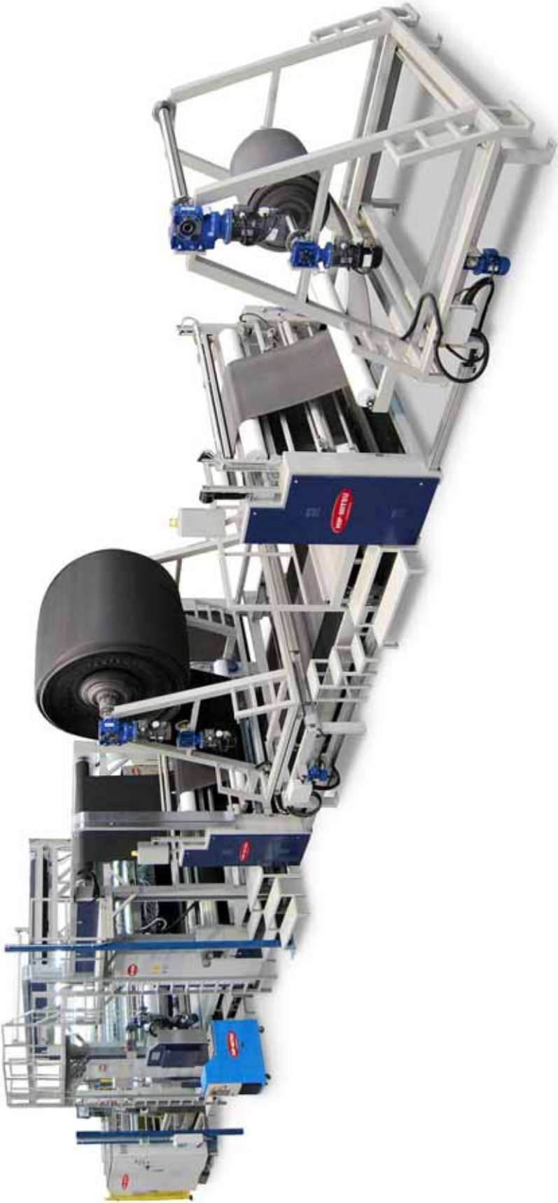
example of three layers converting line for material in roll, included unwinders, web-guide system, slot die, two calender, winder, floor and bridge path, motorized belt. Suitable for insulation and building converter and more...
