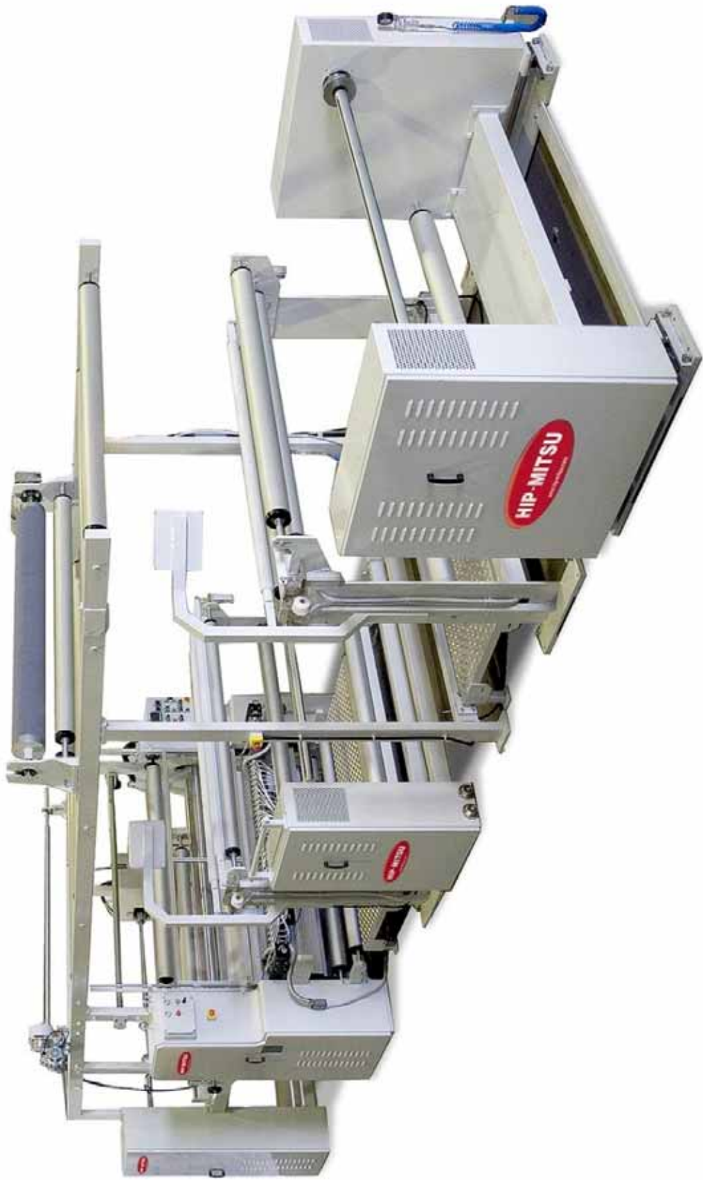
example of two layer converting line for material in roll, included two unwinder, web-guide system, slot die, calender, winder, floor and bridge path; web tension control: traditional. Suitable for automotive, shoes, textile, furniture converter and more...
