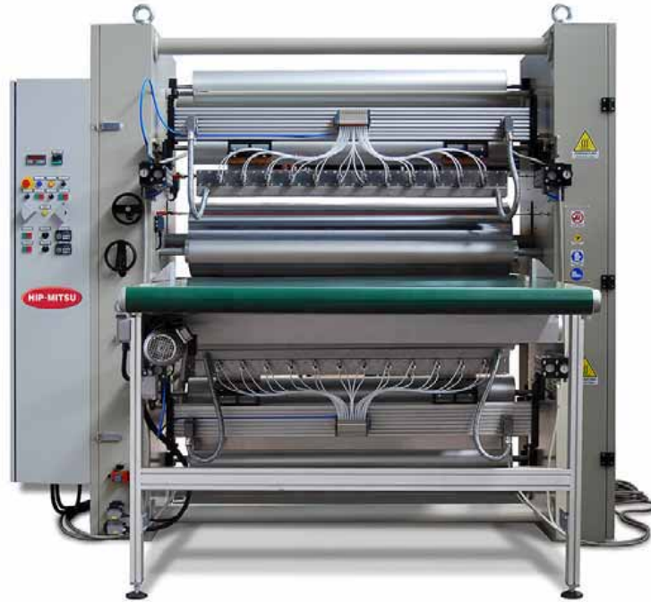
three layer roll to roll or roll to sheet hot melt laminator
